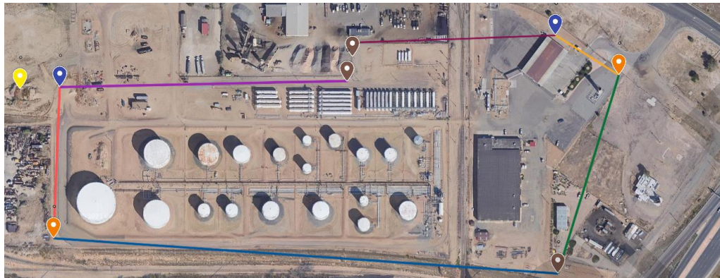
Figure 1: Approximate Layout of the Open-Path Analyzers, Retroreflector Locations, and Meteorological Station
