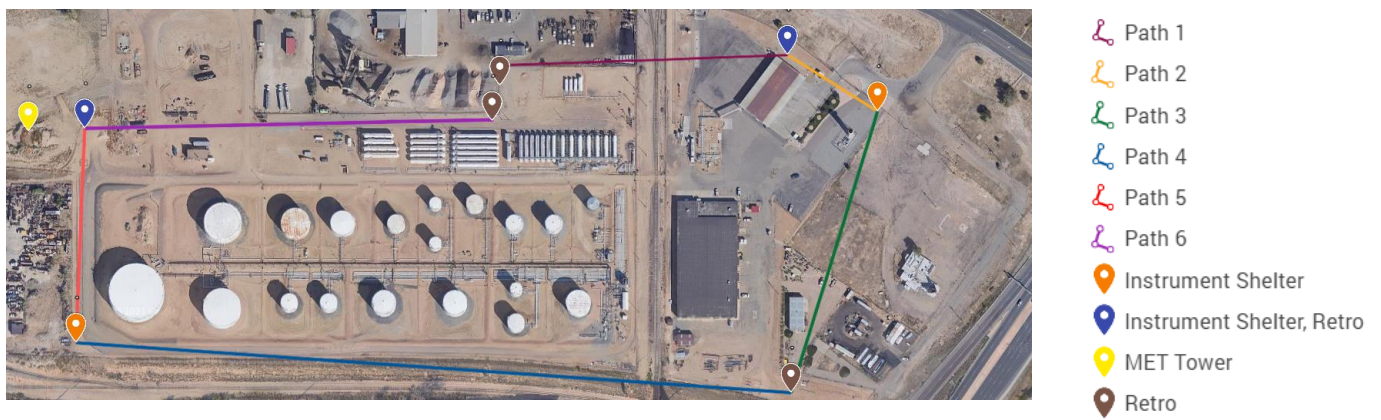
Figure 3-1. Approximate Layout of the Open-Path Analyzers, Retroreflector Locations, and Meteorological Station
